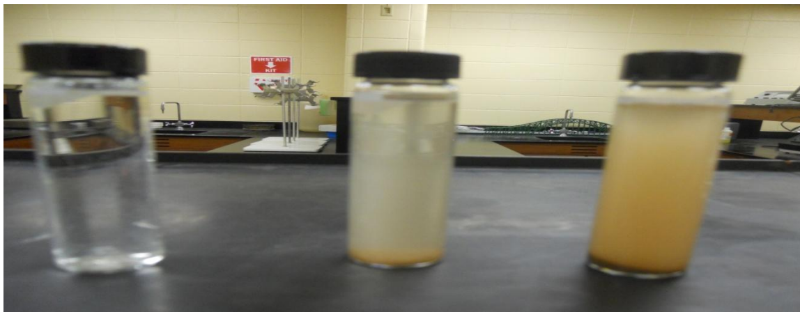
Figure 1: Jars of different turbidity values 0, 250, and 1100 NTU from left to right
